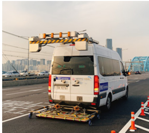
(c) Ground-coupled GPR
